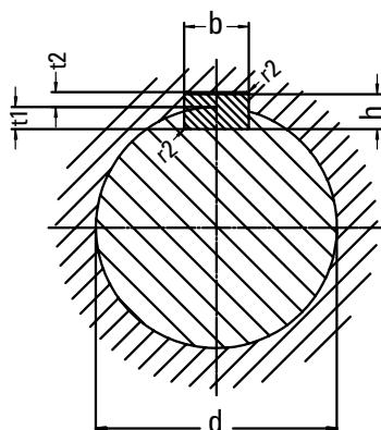
The given values for the bores are valid according to DIN6885-1. As a matter of principle, every key connection must be checked with regard to surface pressure. Keyways according to BS 46, ANSI B17.1 or other standards are also possible. For other types of connections, such as e.g. spline connections in accordance with DIN5480, multiple splined shaft connections, or shrink disc connections, please get in contact with our Technical Department.
