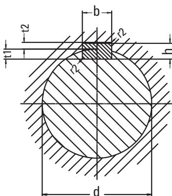
The given values for the bores are valid according to DIN6885-1. As a matter of principle, every key connection must be checked with regard to surface pressure. Keyways according to BS 46, ANSI B17.1 or other standards are also possible. For other types of connections, such as e.g. shrink-fit connections or spline connections in accordance with DIN5480, multiple splined shaft connections, or shrink-fit sleeve connections, please get in contact with our Technical Department.
