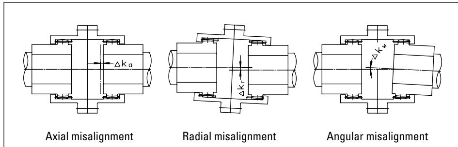
For standard Gear-Couplings the misalignment can be up to  $\pm 0.75^\circ$  per toothed plane. The misalignment values specified are maximum values that cannot be allowed to occur at the same time.
