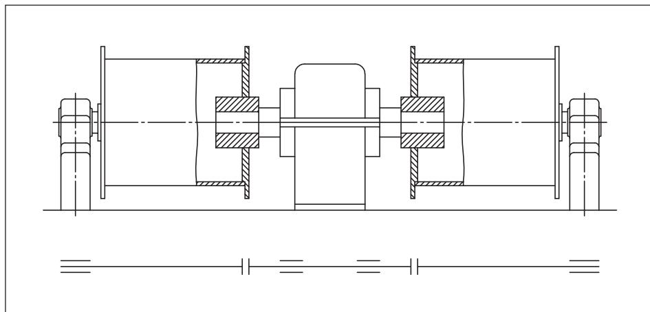
Fig. 1 Layout of a twin drum drive with four-point beared rigid shaft without a Drum-Coupling.
