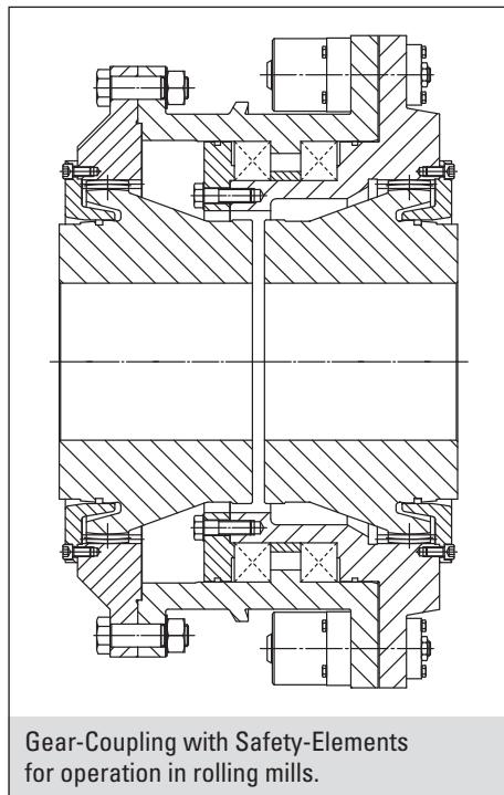
Gear-Coupling with Safety-Elements
