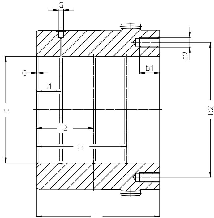
The Gear-Coupling hub must be brought up to the required shrinking temperature  $T$  before assembly.
