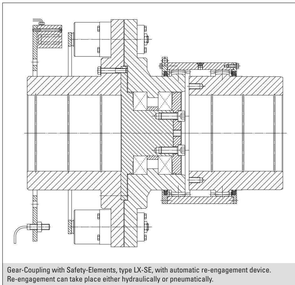
Gear-Coupling with Safety-Elements, type LX-SE, with automatic re-engagement device.
