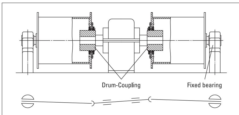
Fig. 2 Layout of a twin-drum drive with a Drum-Coupling.
