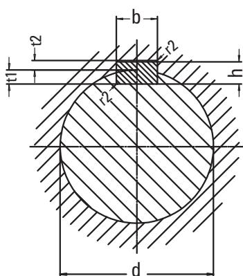
The given values for the bores are valid according to DIN6885-1. As a matter of principle, every key connection must be checked with regard to the surface pressure. Keyways according to BS 46, ANSI B17.1 or other standards are also possible. For other types of connection, e.g. spline connections according to DIN5480 or multiple splined shaft connections, please contact our Technical Department. Shrink-fit connections see next page.
