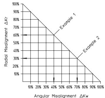
For standard MALMEDI Gear-Couplings of the S-NX series the misalignment can be up to  $\pm 1^\circ$  per tooth ing plane. The misalignment values specified are maximum values that cannot be allowed to occur at the same time. Where there is simultaneous radial misalignment  $\Delta K_r$  and angular misalignment  $\Delta K_w$  these values must be reduced in accordance with the diagram.
